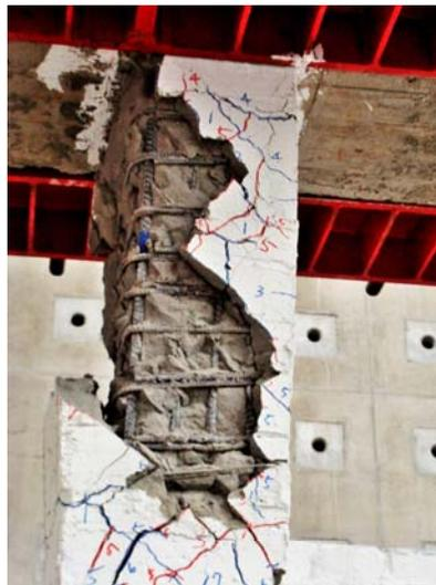
側位移比1.75%，混凝土嚴重崩落
