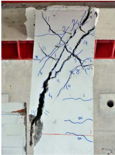
側位移比1.5%，斜向裂縫貫穿短柱
